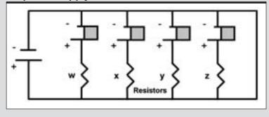
advantage of continued operation of all functioning LEDs even if one or more LEDs fail. In either type of circuit, it is important that the anode and cathode connections be alternated. This is because LEDs have polarity and current will only flow in one direction. Placing two anodes or two cathodes in sequence will disable the circuit.
