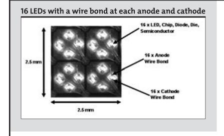
welding or thermal compression is used to electrically connect LED chips to a printed circuit board (PCB). One wire bond is made at the chip's positive terminal or anode while the other is made at the negative connection or cathode.
